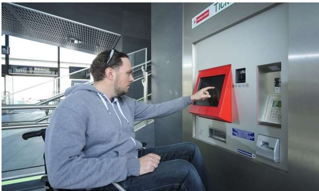
Figure 124: Accessible ticket machines for wheelchair users
