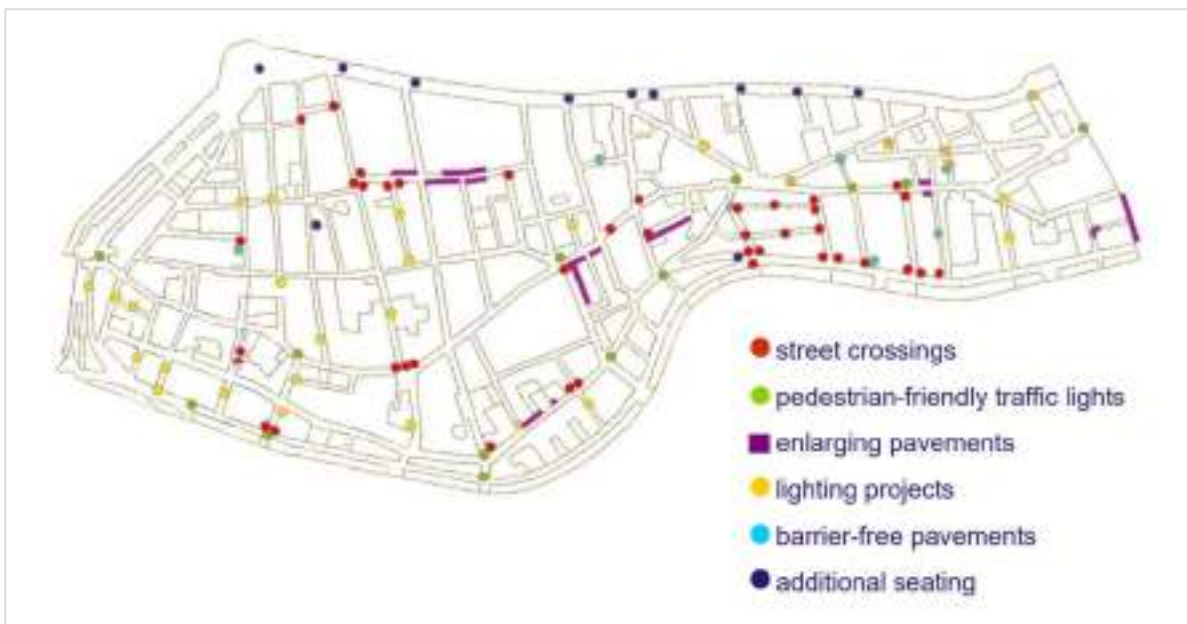
Figure 113: The district of Mariahilf where gender mainstreaming in urban mobility was implemented during 2002 – 2005. The success of which prompted a further 23 districts to undergo assessment for quality deficits in pedestrian networks (adapted from DI Elisabeth Irschik, 2008).
