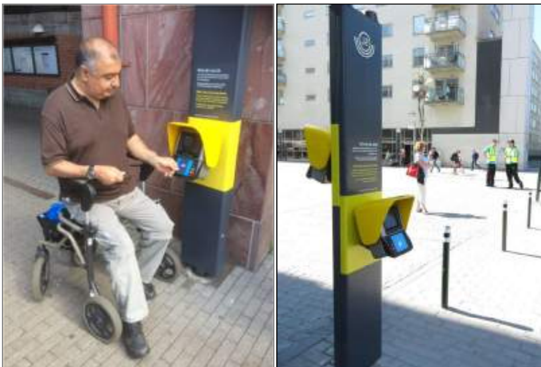
Image 1: The accessible ticket machines are placed at two different heights and used for activating, changing and validating tickets of trains, trams, and ferries throughout Stockholm, but not for purchasing tickets (Trafikförvaltningen Stockholms Läns Landsting).
