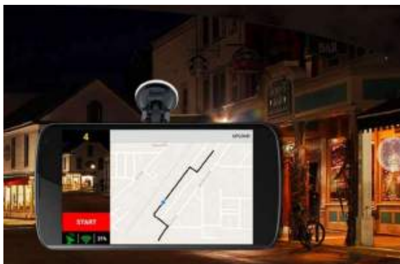
Figure 91: Interface of the Safetipin Nite Application taking photos of the surrounding automatically while mounted to the windscreen of cars (Source: http://safetipin.com/theme-assets/safetipin_common/images/banner-nite.jpg )
